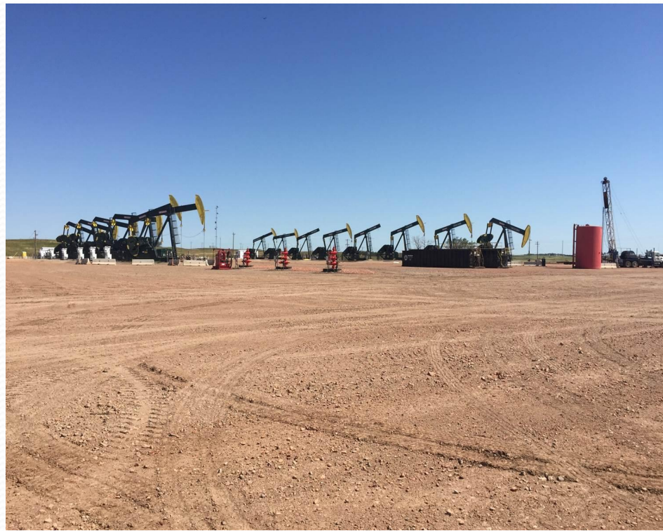
Multi-well Pad: Courtesy of ND Oil and Gas
